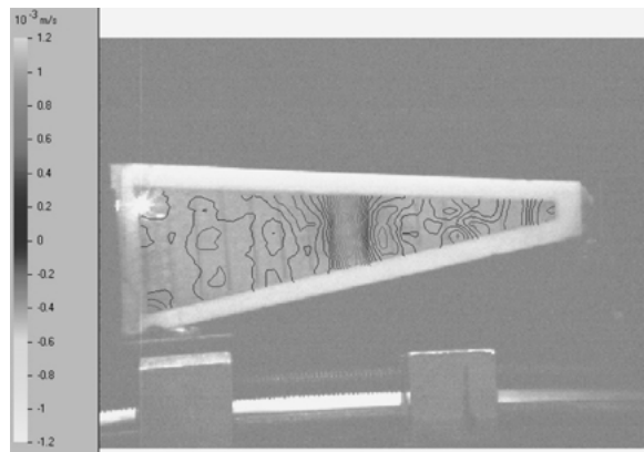
Fig. 18. Laser vibrometer scan of 15-element array segment (element 8 at 45 kHz).
