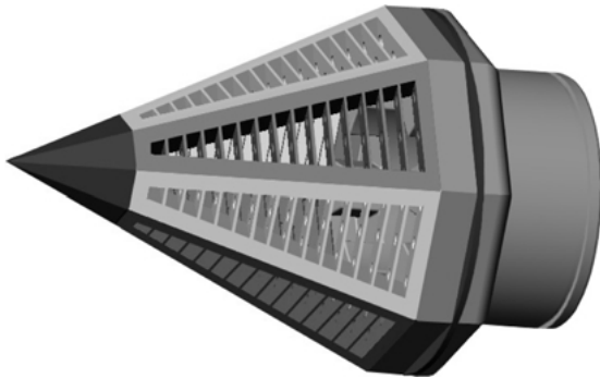
Fig. 15. CAD model of 120-element, conical, octahedral imaging array.
