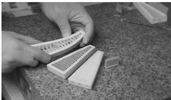
Fig. 16. Three array isolator materials: Shore A60 polyurethane with microballoons (left), Styrofoam (middle), and Shore D80 epoxy with microballoons (right).
