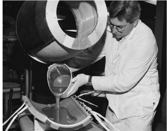
Fig. 10. Application of the absorptive backing (dispensing).
